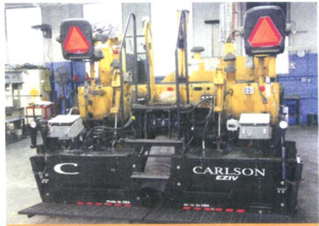
Paving machine with electric screed
